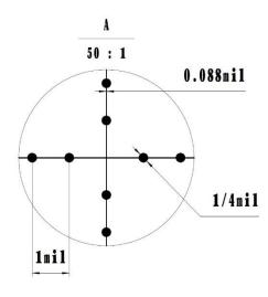
Your new scope has a Mil Dot reticle with matching Mil based turrets. Each click of the turret moves the reticle by one-tenth of a Mil.
